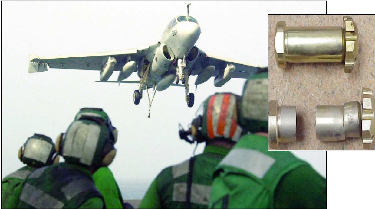
Inset shows arresting wire pin not heat-treated to provide proper strength.
