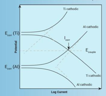
*Figure 1:* Polarization Curve Crossing between the Less Noble Material (Aluminum, Anode) and the More Noble Material (Titanium, Cathode)
