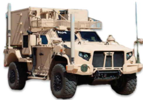
Lightweight Multipurpose Shelter (LMS): a lightweight, transportable, electromagnetic interference-protected, high-mobility multipurpose wheeled vehicle-mounted tactical rigid wall shelter. LMS is the replacement for the S-250 communications-electronics shelter.
