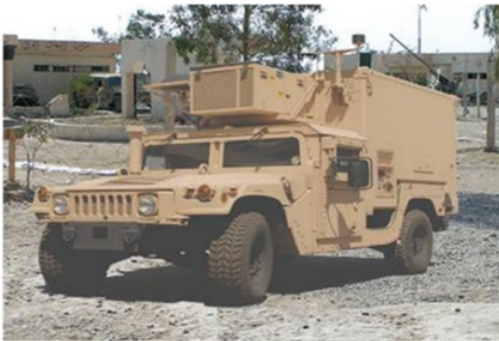
Lightweight Multipurpose Shelter (LMS): a lightweight, transportable, electromagnetic interference-protected, high-mobility multipurpose wheeled vehicle-mounted tactical rigid wall shelter. LMS is the replacement for the S-250 communications-electronics shelter.
