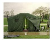
Description: The Small Unit Shower (SUS) is a lightweight, rapidly deployable shower for small units and/or forward deployment. It consists of an air beam supported tent with four stalls with individual hand-held nozzles and water collection basins, and a diesel/JP8 fired water heater that uses 28VDC electrical power from a vehicle slave connection. It comes in three man portable bags that easily fit in a HMMWV bed.
