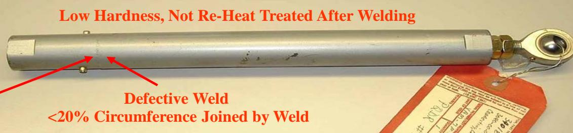
Low Hardness, Not Re-Heat Treated After Welding
