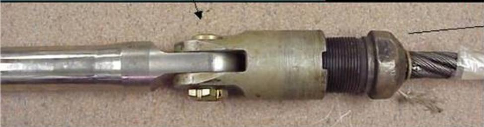
Pin not heat treated to provide proper strength.....
