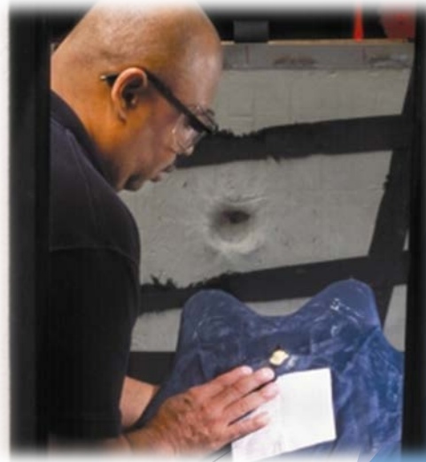
Resultant Behind-armor Backface Deformation
