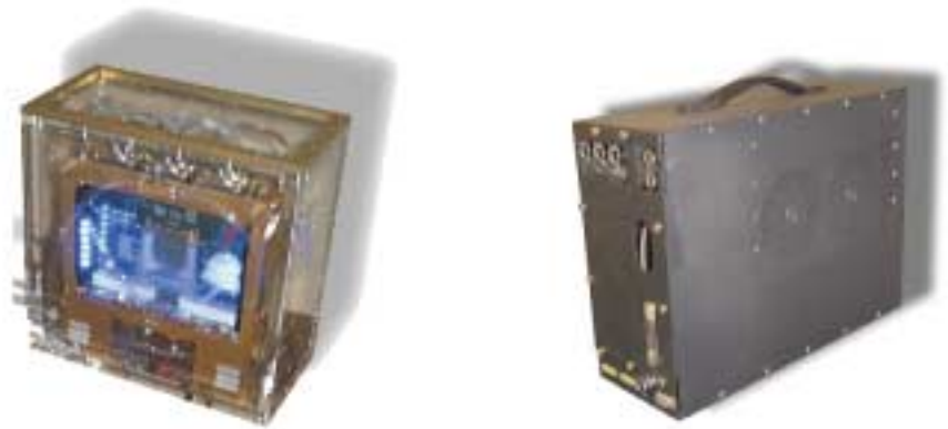
FIGURE 4. Portable Spray-Cooled Laboratory Unit.
